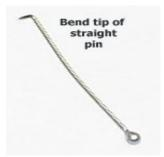
A pair of needle nose pliers or flat nosed pliers will do this job nicely. Bend about 3/32 of an inch 90 degrees. If the bent part is too short or too long, it won't work as well.
