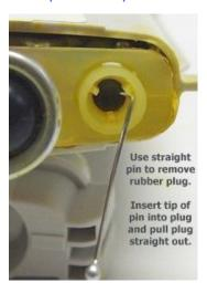
Start pin into plug with pin horizontal. As you get the tip started into the plug, straighten the pin so it is vertical. Make sure the tip of the pin is firmly inserted into the plug. Then, gently pull on the pin and the plug will come out. Try not to damage the plug too much, it can be used again if not damaged.
